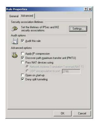
At this stage we've completed SSH Sentinel configuration and we are ready to perform a diagnostic test. Click OK to go back to the SSH Sentinel Policy Editor window and click "Apply" to update security policy changes we've made.
